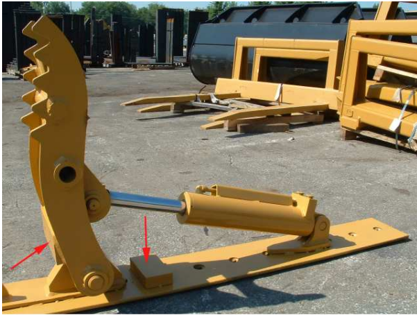
90 degree position of thumb. Note stop blocks.
