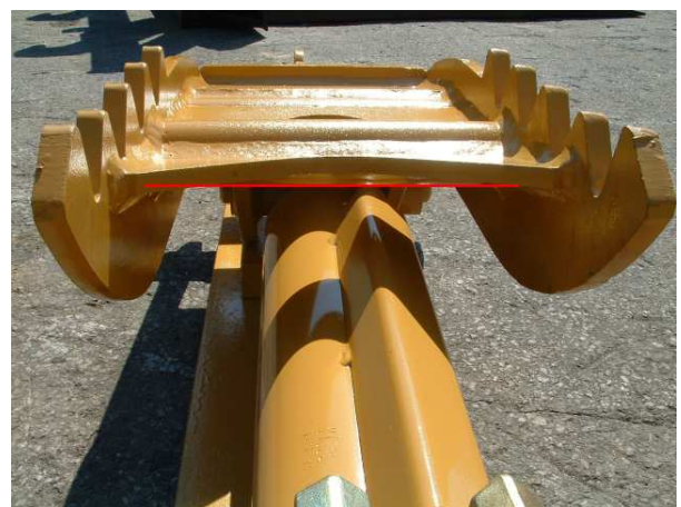
Clearance of thumb and cylinder when stop is properly used.
